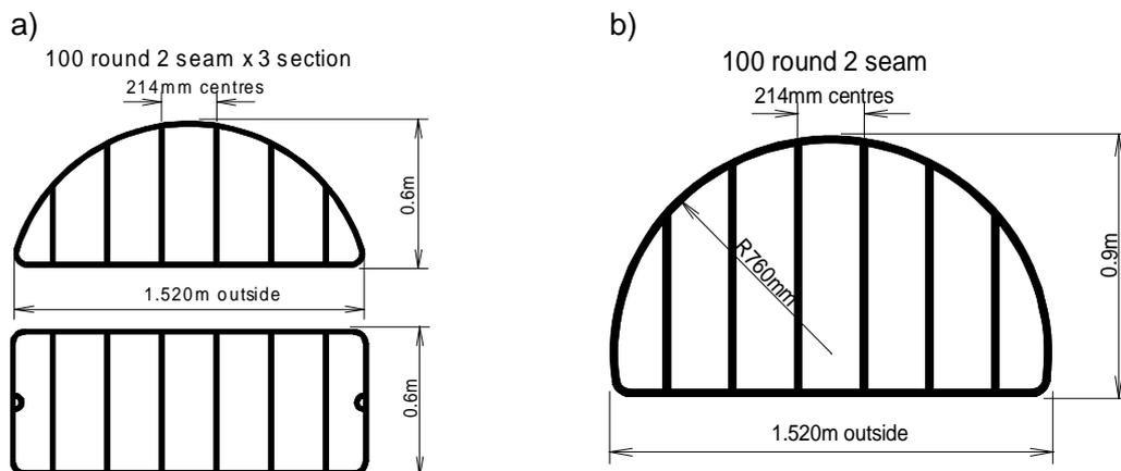
**Figure 1. Design of the SED prototypes to be used with mesh hoods on the SESSF wet boats a) three section SED; b) two section SED.**
