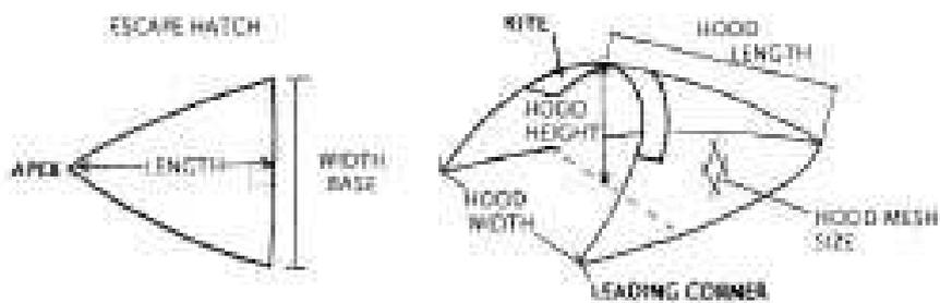
Figure 1. Diagram of a generalised SED showing the terms used to describe the different parts of the SED, including grid and escape hatch specifications (from Cawthorn).
