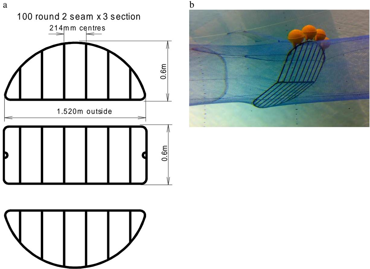
Figure 2. a) Design of the Motnets SED (note: mesh hoods were used with this design); b) image of a bycatch reduction device in a flume tank similar to that being developed as a SED for the SESSF wet boat fleet.
