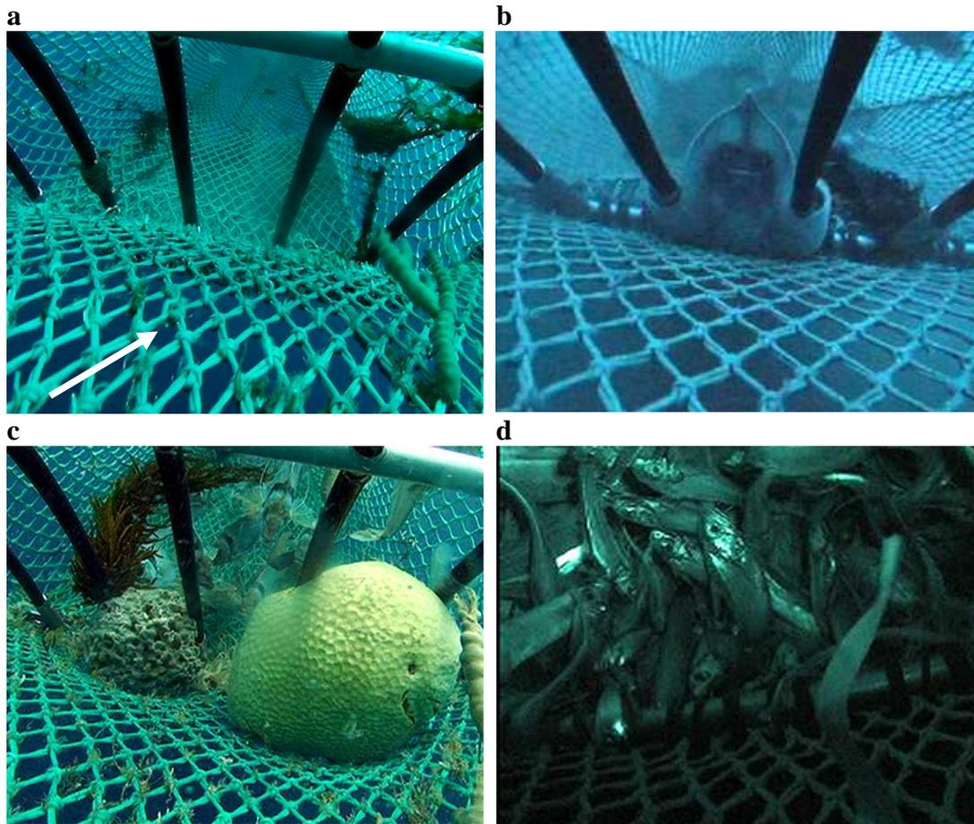
**Figure 8.** Images of the Bennett SED from the underwater video taken during 2nd sea trial showing: a) the SED sitting with the floor of the net ballooning up; b) a skate caught on the bottom of the SED; c) sponge accumulating at the base of the SED rather than going out through the escape hatch; and d) blue grenadier and other fish clogging up the SED.
