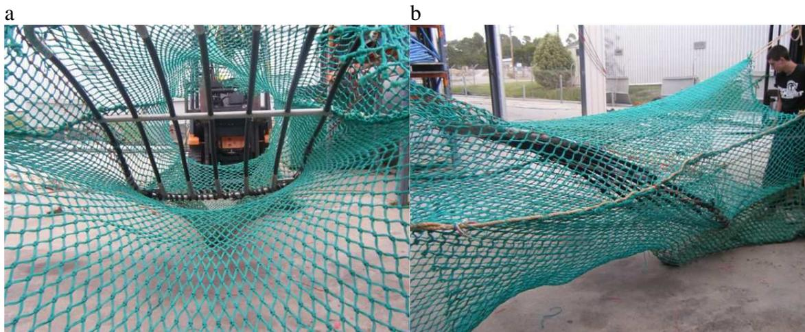
**Figure 5.** Position and installation of the Bennett SED in the net of the Western Alliance view from a) forward of the SED and b) at the side, showing the slight curve of the SED.
