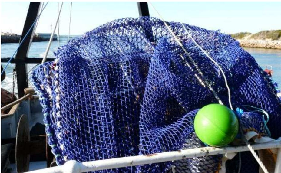
**Figure 7. Protruding Motnet SED wrapped around the net drum.**
