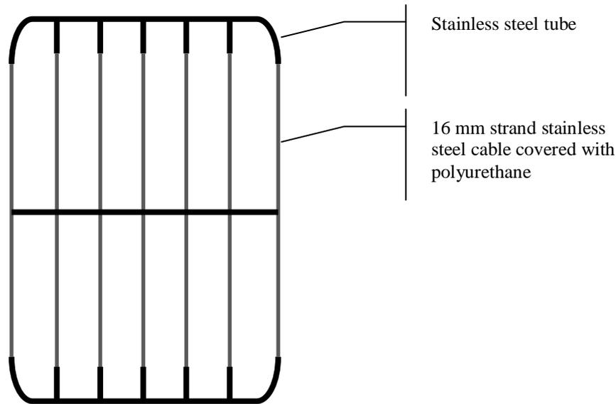
**Figure 4.** The construction of the Bennett SED, trialled on the Western Alliance. The escape hatch was positioned on the underside of the net to aid the removal of large rocks, rays and sponge as well as seals.
